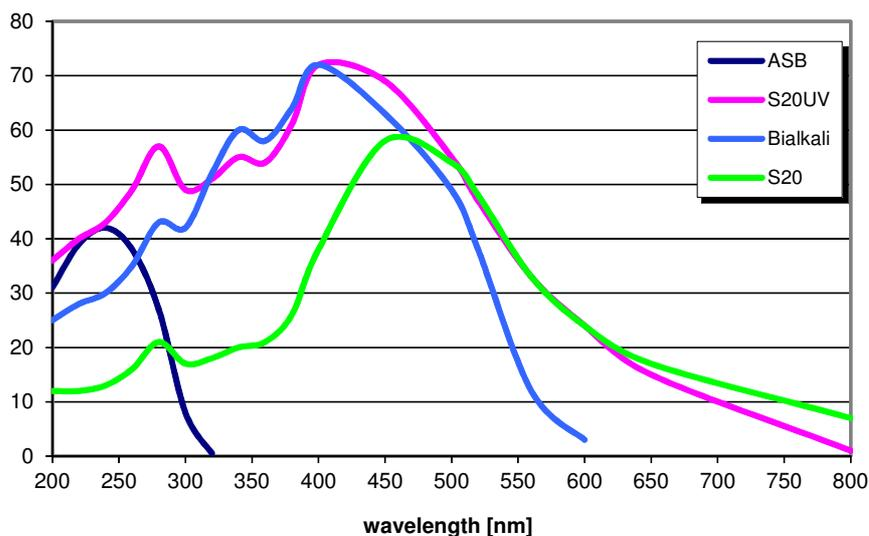
The sensitivities (in mA/W) shown above refer to non-gateable photocathodes on a quartz substrate.
